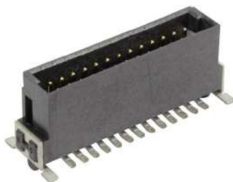
Figure 12: 26 pin IDC connector found in the PCO-170T800 [Harting]
