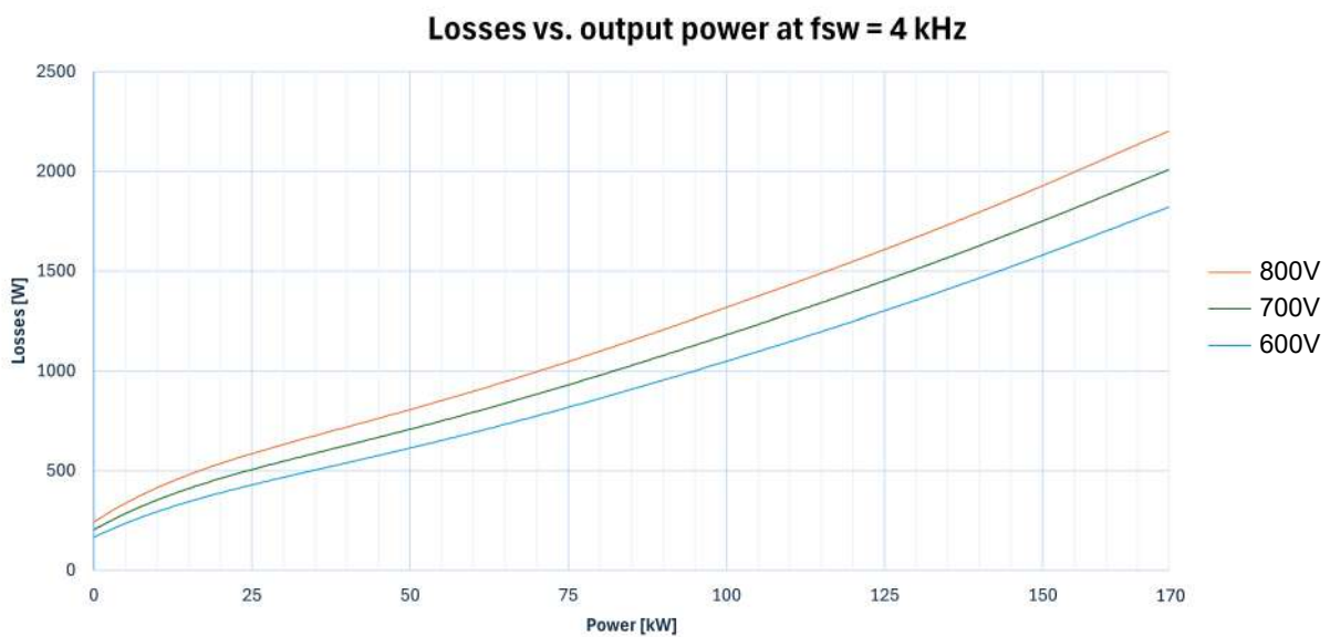
Figure 10: Losses vs. output power at a switching frequency of 4 kHz
