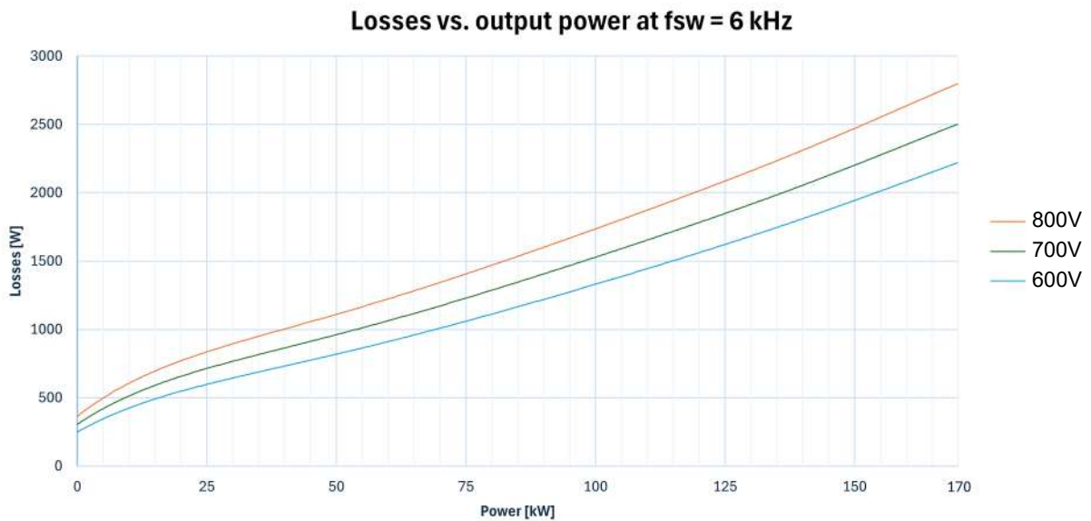
Figure 9: Losses vs. output power at a switching frequency of 6 kHz
