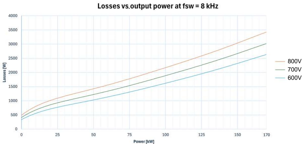
Figure 8: Losses vs. output power at a switching frequency of 8 kHz
